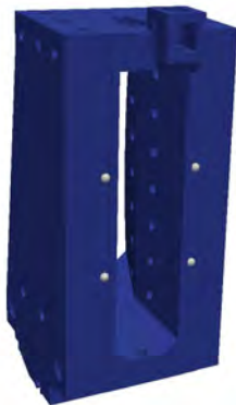
CAD model with mounting points determining the TCP location
